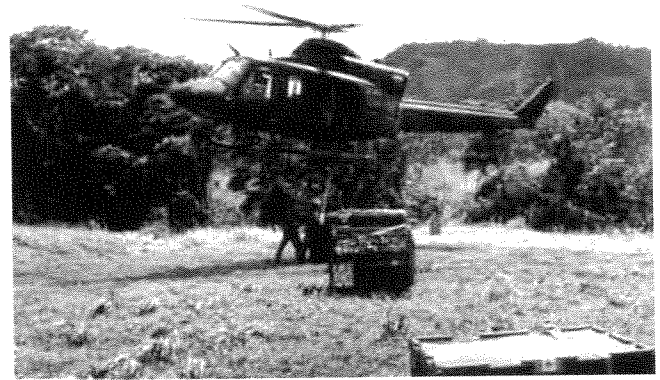
Water slinging of bagged water by CH-146 Griffon for delivery to isolated communities.
