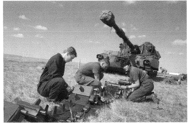
Ex Prairie Ram 13 to 26 May 98 - Gnr Nicole Coxworthy, Gnr Thomas Douglas, Gnr Laura McKenzie replacing track.
