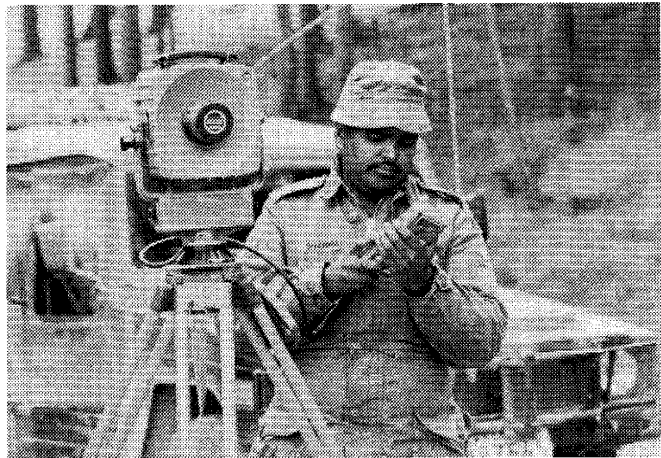
Bdr D.M. Sharma operates MRA-7 Tellurometer, Grafenwohr, Sept 91.
