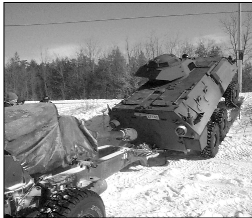
Figure 9: GRIZZLY/LG1 negotiating 20 Degree Slope.
