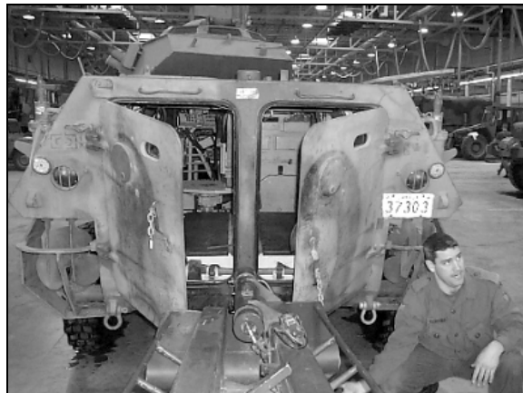
Figure 11: Doors contacting with spades at 0 degrees.
