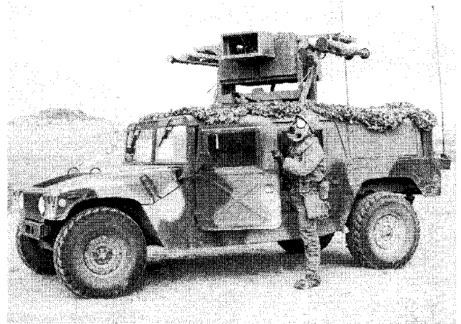
SETTER: US Army Missile Command proposal for PMS. Spike rockets would be mounted in clips in the centre of the pedestal.
