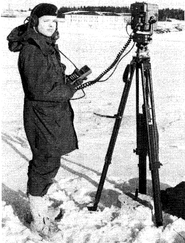
Bdr Gillis demonstrates the MRA 7 Tellurometer in preparation for the trial in early 1986.
