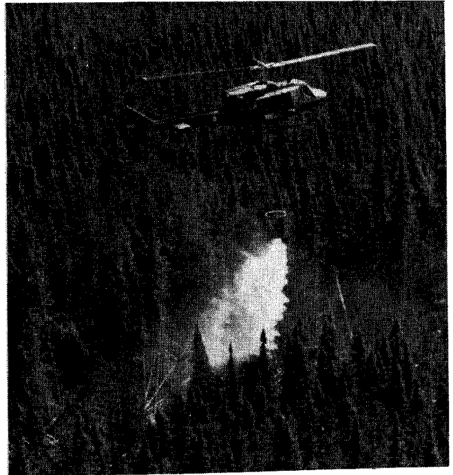
Water bucket-equipped Huey. Due to the smoke appearing downwind from the fire, FACs were required for accurate water drops.
