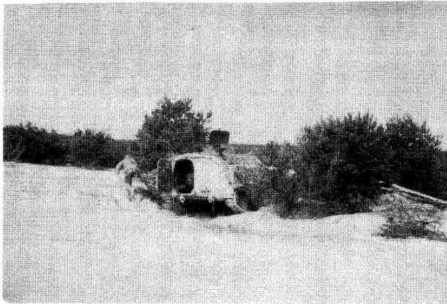
RATAAC on AMX 10. Bde level surveillance radar also used to adjust artillery. Found in Radar Section of Communications Troop Close Support Regiment.
