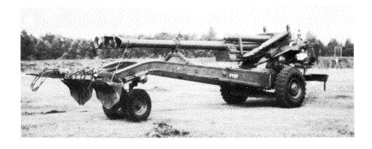
The new 155mm howitzer FH 70 in the self-propelled position, with auxiliary wheels lowered. The maximum range is 24 km, but this will increase to 30 km when rocket-assisted rounds are developed.
