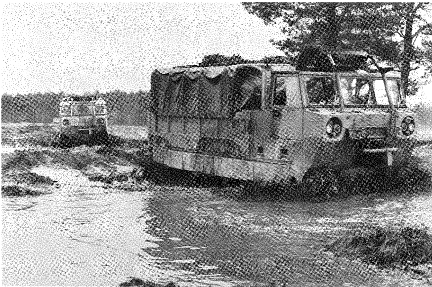
C Bty M 548s swim after the guns during February firing practice.
