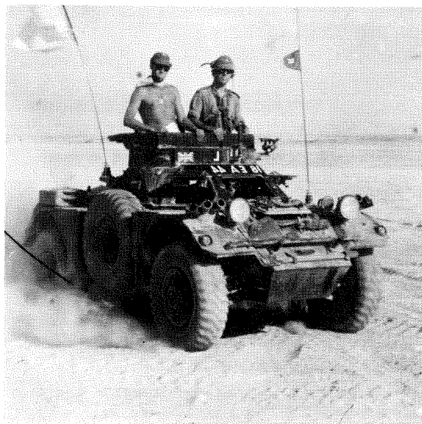
Even routine moves required the use of the sun compass, shown mounted on left side of turret, for desert navigation as land marks were very scarce.
