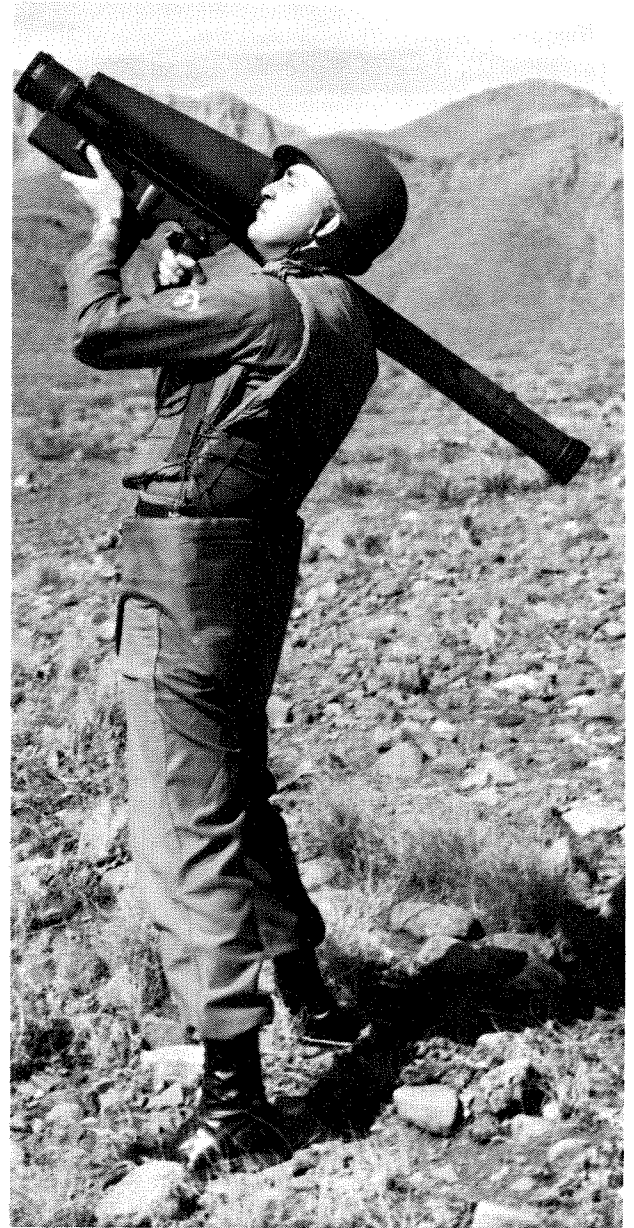
Redeye - This system consists of a missile sealed in a launcher approximately four feet long and three inches in diameter. The missile can only be removed by firing. Stabilized by four rear fins and steered by two movable fins in front, the missile has an IR homing guidance system.
