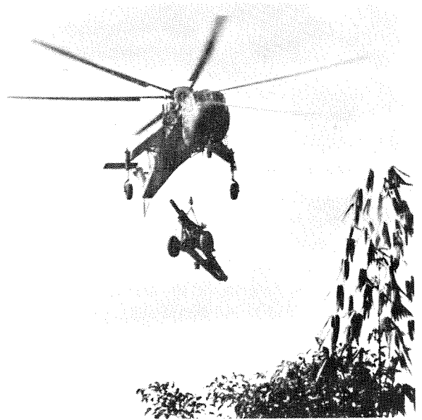
By airlift, that's how — giant skycrane lifts a 155mm howitzer to a new position.
