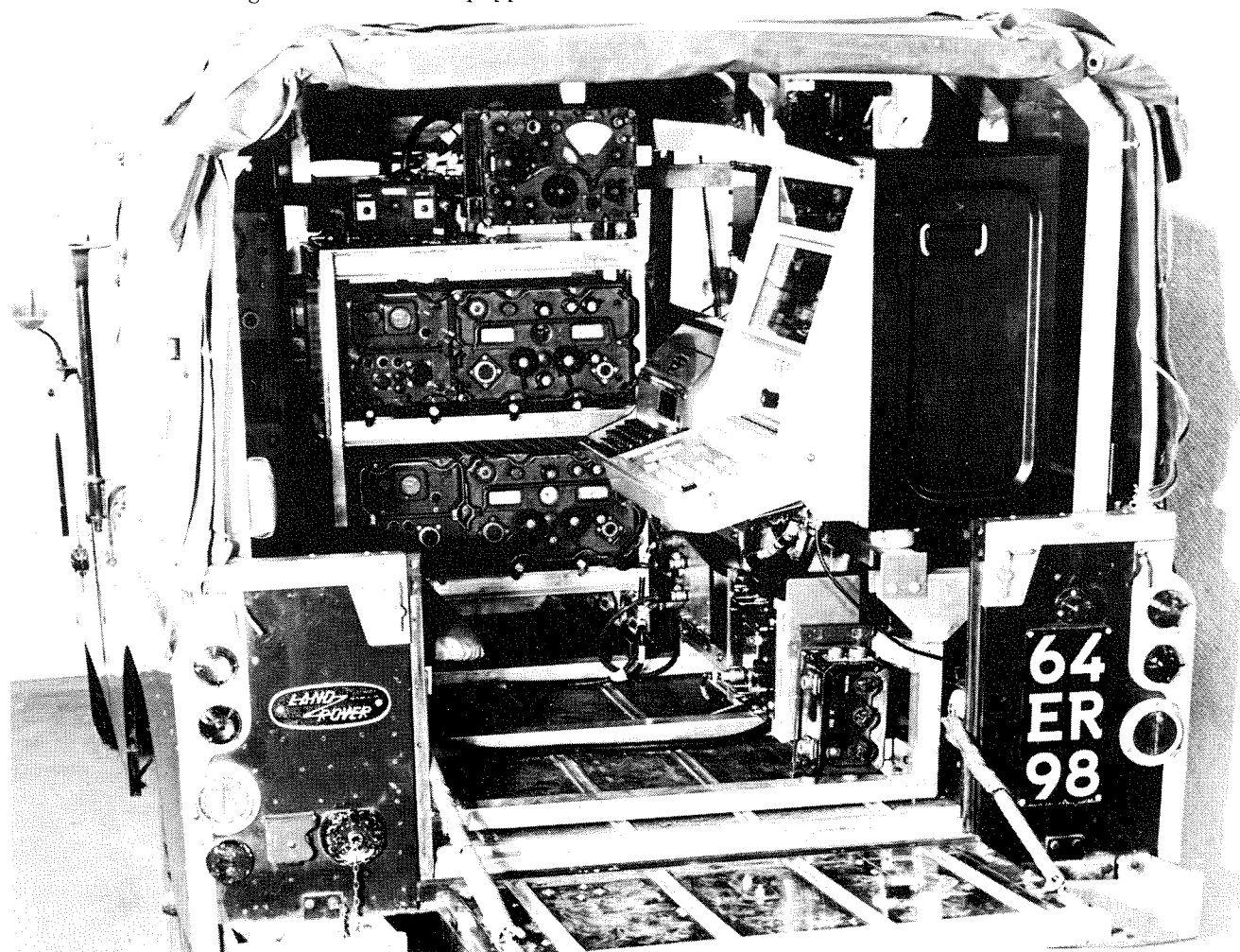
FACE mounted in the ¾ ton Land Rover showing the battery command post installation.
