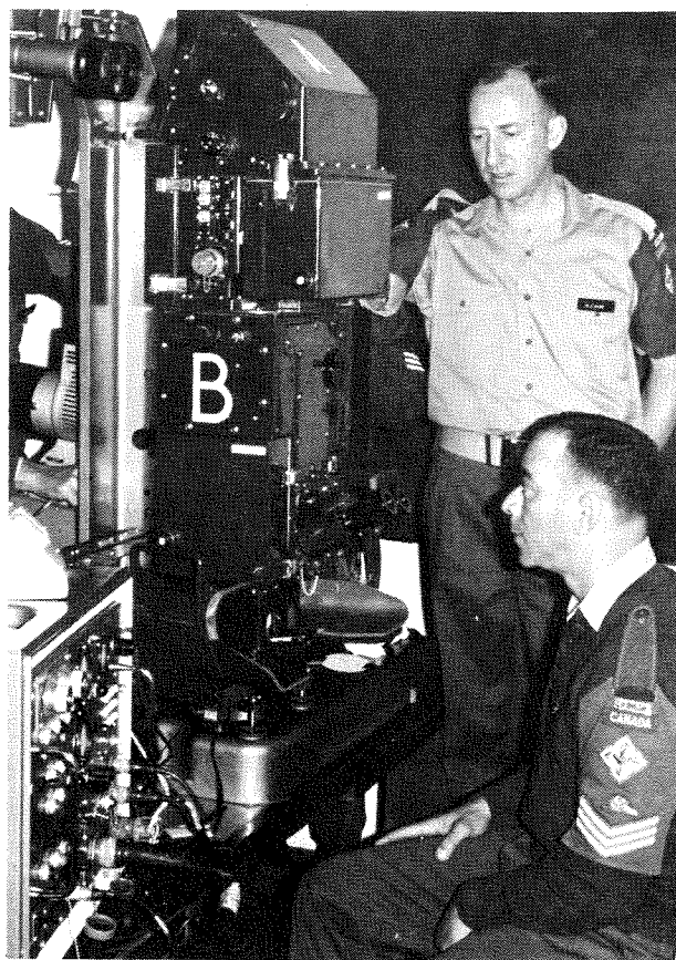
The Rapier Tracker is fixed to an aircraft simulator training aid for the training of tracker operators on aircraft tracking drills. Pictured are MWO Rice and Sgt Bell of the Canadian Rapier Trials Team.
