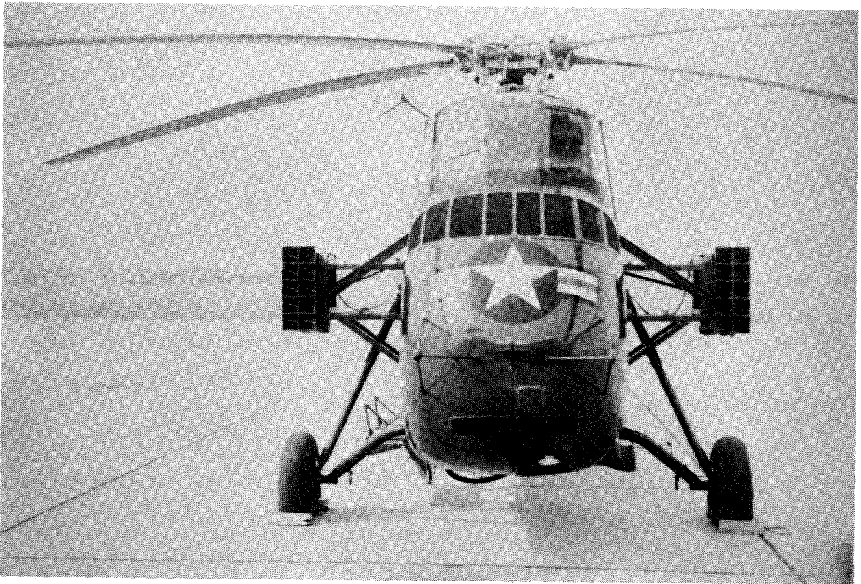
CH-34 Helicopter mounting twenty - 4.5 inch Rocket Tubes, ten on each side of aircraft.
