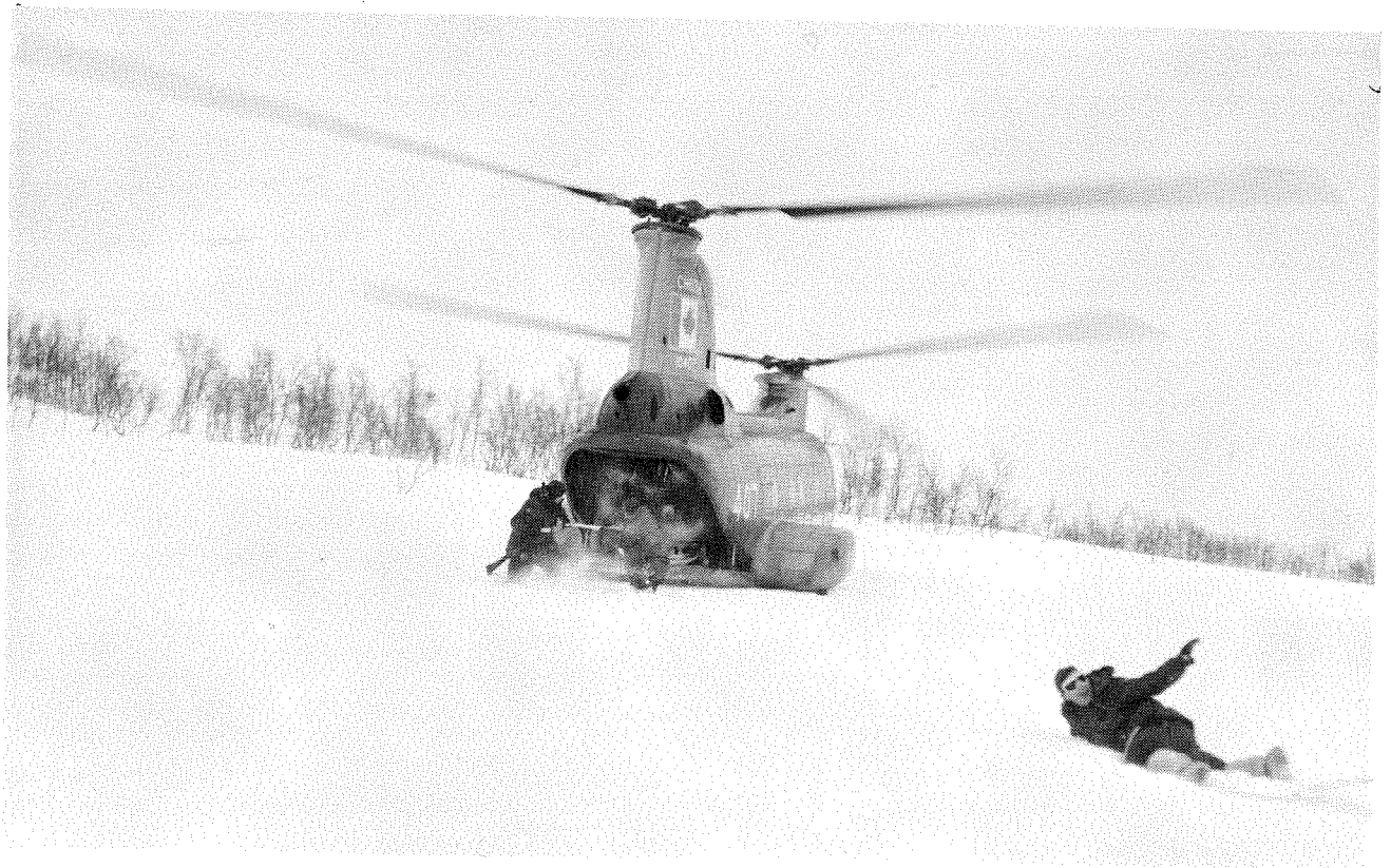
Mortar detachment dismounting from Voyageur. The depth of snow often prevented the ramp from opening fully, and the effort of loading and unloading was further aggravated by propellor driven snow which sometimes reduced visibility to a few feet
